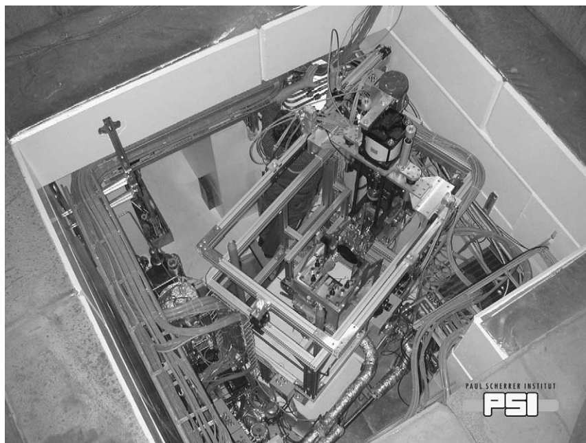
Fig. 19. Photo of the LiSoR loop installed in the IP1 bunker.
