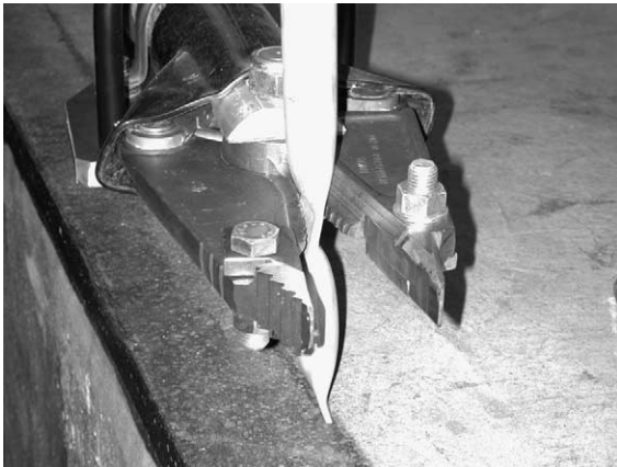
Fig. 15. Hydraulic squeeze and cut device for disconnecting the LBE pipes of the test section from the loop. The front part squeezes the pipe and the back part of the device cuts the pipe.
